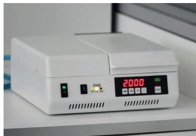
Fig. 2 Otofash G171 – post-curing 2000 flashes
