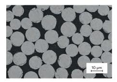
Fig. 2: SEM image (magnification 2kx) of a cross-section of 3M™ RelyX™ Fiber Post 3D Glass Fiber Post. Glass fibers are depicted as white spots surrounded by a composite resin matrix. Source: 3M Oral Care internal data.
