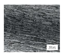
Fig. 7: Surface of 3M™ RelyX™ Fiber Post 3D Glass Fiber Post (SEM, 200x magnification). Source: Peez et al.<sup>2</sup>
