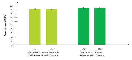
Fig. 6: Pull-off bond strength values of 3M<sup>™</sup> RelyX<sup>™</sup> Ultimate Adhesive Resin Cement and 3M<sup>™</sup> RelyX<sup>™</sup> Unicem 2 Automix Cement in comparison. Both materials show same performance in light-cure (LC) and dark-cure (DC) mode. Source: Peez et al.<sup>2</sup>
