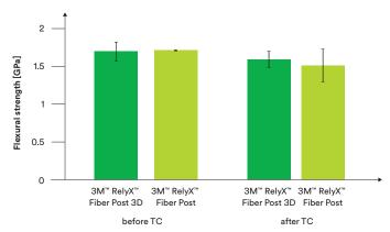
Fig. 5: One-point flexural strength testing before and after thermocycling (TC), 10,000 cycles, 5 °C/55 °C, dwell time 30 s, change time 8 s. Source: 3M Oral Care internal data. Data available upon request. See last page for contact information.
